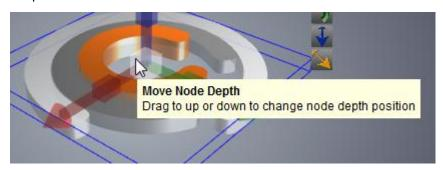
6. When we can't move the shape with manipulator, we can switch to the "Shape" tab, and change Z value for the position.
